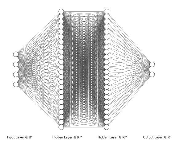
Figure 3.2: A neuron architecture architecture with input 4 node, two dense full connected layers 24 nodes, and 2 nodes at the output
