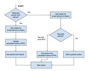
Figure 4.3: Flow of using broad-persistent advising. The agent will reuse previously obtained advice with 80% chance (decays over time) and perform its exploration policy for the remaining change (20%).
