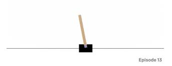
Figure 3.1: A graphical representation of the Cart Pole environment. The goal is to keep the pole balanced while applying forces to the carriage. The terminal condition is that the pole deviates more than 12 degrees from the vertical or the wagon moves 2.4 units from the center.
