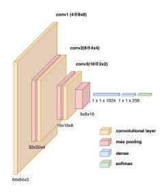
Figure 3.4: CNN architecture with 64x64 RGB image as input, group of three convolution layers, three max-pooling layers, two dense full connected layers, and a softmax function at the output
