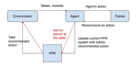
Figure 4.1: Process flow of an interactive reinforcement learning agent using PPR system. After receiving advice from the trainer, the agent will store the action into the PPR model. In the iteration not receiving advice from the trainer, the agent will check and reuse the old advice (red arrows) from the past.
