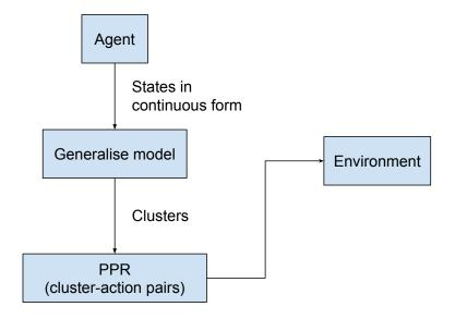
Figure 4.2: Broad advice transform continuous states into finite clusters. Hence, the stateaction pair becomes cluster-action used in the PPR model.
