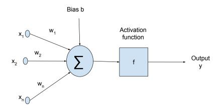
Figure 2.3: The simple architecture of a neural network. Neural network tries to transform from a screenshot image into the next action need to perform for playing Mario game automatically.
