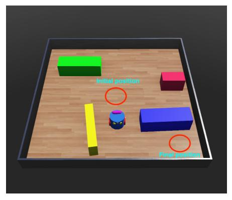
Figure 3.3: A example of Webots environment with initial position and final position. The robot has goals to go from initial position to final position while avoiding obstacles. The robot will be returned to its initial position after any collision.
